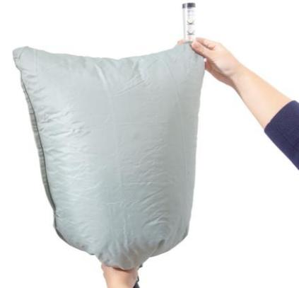
**2.3** Place the face shield in the flow meter bag and start the fan.
