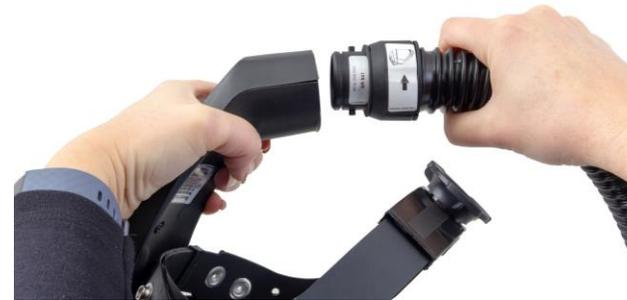
**1.3** Connect the hose to the fan unit and turn it clockwise about 1/8 of a turn.
