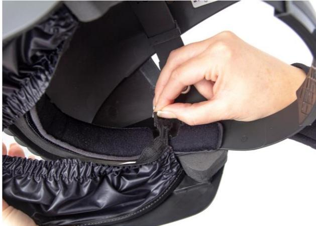
**6.1** Release the face seal hooks from the head harness.
