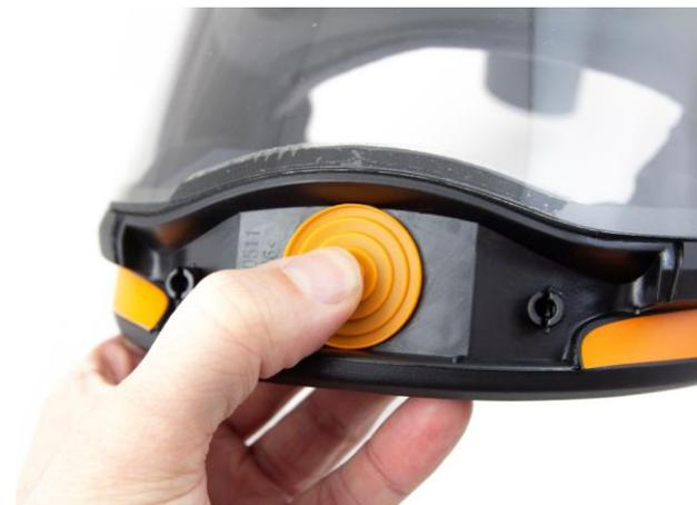
**7.4** Press the new membrane onto the pin. Carefully check that the membrane is in contact with the valve seat all way round.
