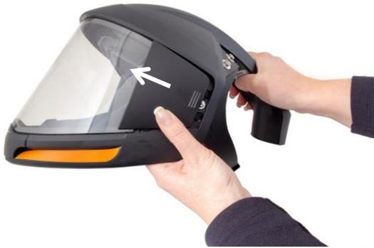
**4.2** Release the visor by moving the lever of the over-centre lock upwards through about 180 degrees. And remove the visor.
