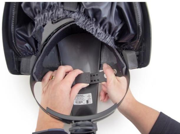
**3.2** If necessary, adjust the head harness in height by lengthening or shortening the strap for the top of the head
