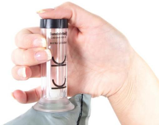
**7.1** Cause a flow stoppage by still holding tightly the joint between the hose and the flow meter bag and then blocking off the flow meter outlet.
