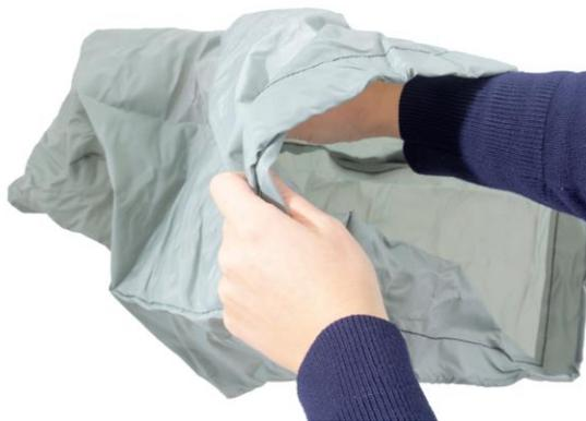
**6.2** Turn the flow meter bag inside out so that the transparent measuring tube is on the outside.
