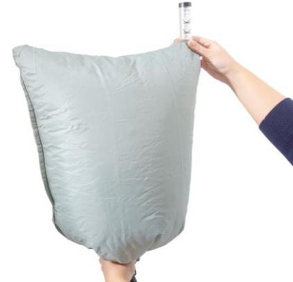
**6.3** Place the head top in the flow meter bag and start the fan unit.
