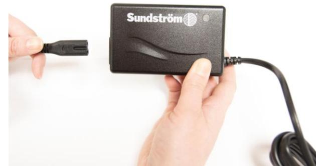
**1.3** Connect the power supply lead to the battery charger. Connect the battery to the battery charger. Connect the power supply lead of the charger to the wall socket.
