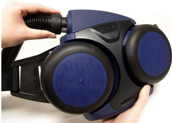
**6.1** Check that the fan is complete with filters, is correctly fitted, cleaned and undamaged.
