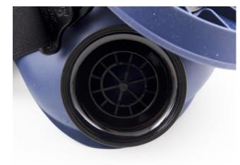
8.2 Critical areas are the exhalation membranes and the membrane seats which must have clean and undamaged contact surfaces. Inspect all parts and replace with new parts as necessary. Leave the mask to dry, and then assemble it.
