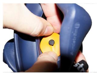
**5.2** Check the edge of the inhalation valve. Gently stretch the flap until it slips over the stud.
