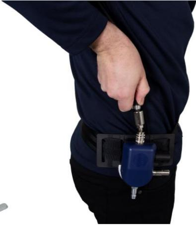
**2.4** Connect the breathing hose of the compressed air attachment to the control valve outlet.
