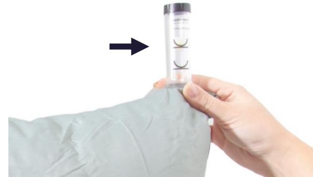
**1.5** Read the position of the ball in the tube. It should float level with or just above the marking on the tube.
