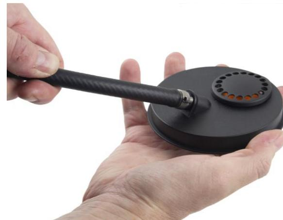
**6.4** Apply a load to the hose to check that it is firmly secured to the adapter.
