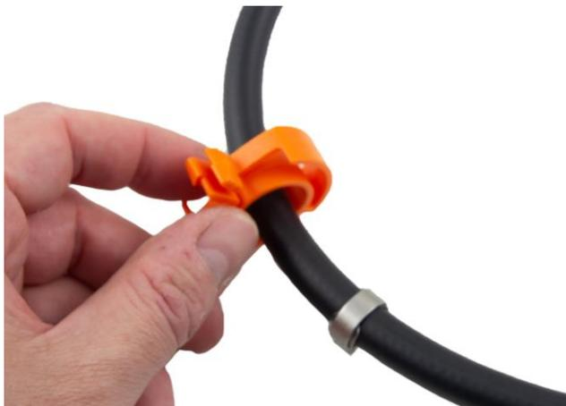
**6.2** Thread the hose clip and retaining clip onto the new hose.
