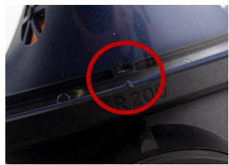
12.4 Markings are made to show the centres of the visor, frame halves and mask. Press the new visor into the groove, making sure that the centre markings are in line. To make assembly easier, coat the slot with a soap solution or similar liquid.
