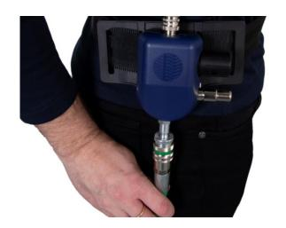
**10.1** Disconnect the compressed air hose from the control valve.
