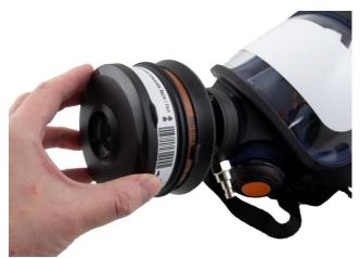
**3.4** Turn the filters into the face piece. Screw until the thread reaches the seal at the bottom of the filter connection, then another 45 degrees.
