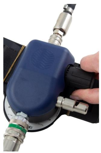
**8.1** Use the control valve knob to set the air flow rate to suit your current work intensity. Fig. 3. In the fully closed position (turn the knob anti-clockwise), the flow is about 150 l/min. In the fully open position (turn the knob clockwise), the flow is about 320 l/min.
