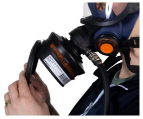
**9.1** Remove the sealing cover, if fitted.
