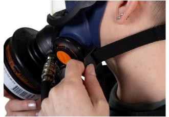
**9.3** Slacken the four elastic straps in pairs by moving the strap holders forward. The two inelastic straps need not be released.
