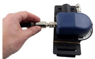
**1.4** Check that the air flow - measured through the mask - is at least 150 l/min.
