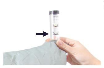
**2.2** Read the position of the ball in the tube. It should float level with or just above the marking on the tube.
