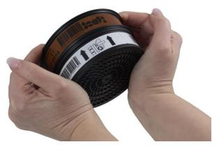
3.1 During work in atmospheres containing both particulates and gases/vapors (such as spray painting) the particulate filter and chemical cartridge should be combined. Press the filter/cartridge together so that the arrows on the particulate filter point towards the chemical cartridge.
