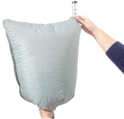
**2.1** Place the facepiece in the bag and grip the opening of the bag so that it seals around the breathing hose. Grip the flow meter with the other hand and hold it so that it points vertically up from the bag.
