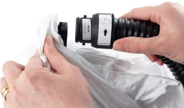
**6.3** Fit the new hose into the head harness in the reverse order. One hose connection is fitted with an O-ring. This end should be connected to the fan/compressed air unit.
