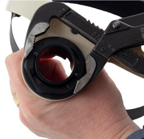
7.3 Turn the locknut a quarter of a turn to remove it. Use polygrip pliers if the locknut is stiff to turn.
