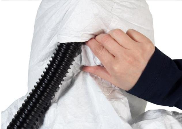
**3.4** If necessary, adjust the circumference of the head harness by means of the knob at the rear of the head harness. The knob is on the inside of the hood behind the hose. You can reach it without taking off the hood. Turn clockwise to tighten and counterclockwise to widen.
