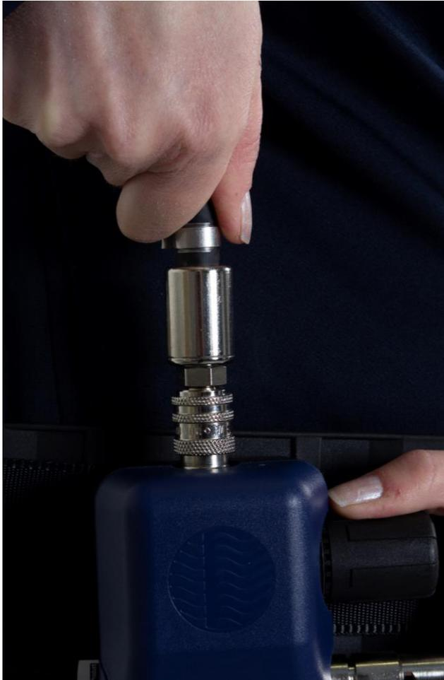
**9.1** Both couplings are of safety type and are released in two stages.
