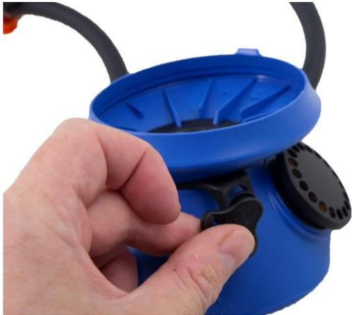
**11.1** The head harness can be ordered as a spare part only as a complete harness. Snap the strap holders of the head harness off the mask strap mountings.
