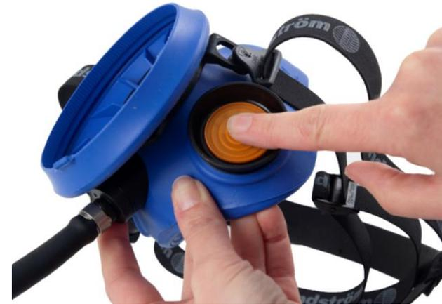
**10.3** Press the new membranes onto the dowels. Carefully check that the membranes are in contact with the valve seats all round.
