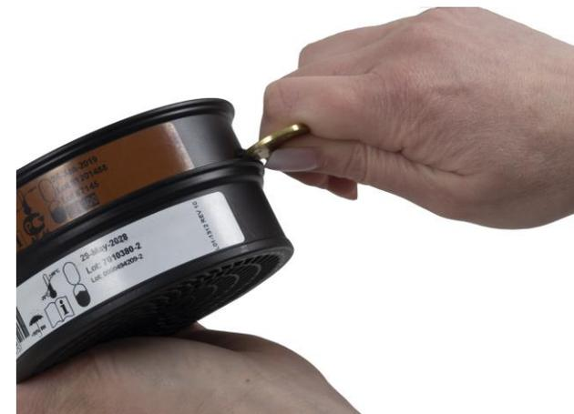
**3.4** To separate a combined filter, place a coin in the space between the lower lip of the particle filter and the small tab molded into the side of the gas filter. Push firmly and twist the coin until the filter pops off.
