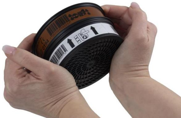
**3.2** Place the particle filter on top of the cartridge. Grasp both protective elements. Squeeze hard until you hear the particle filter snap onto the gas filter.
