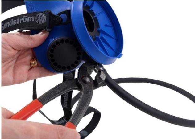
**12.1** Cut off the hose clip with a pair of pincers and pull the hose off.
