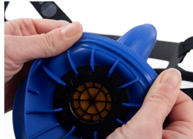
**1.3** Carefully check that the internal groove of the mask is clean and undamaged.
