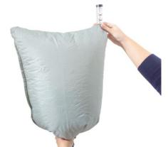
1.6 Place the head-top in the flow meter. Grip the bag to seal around the breathing hose. Grip the flow meter tube with the other hand, the tube will point upwards from the bag
