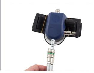
**1.3** Connect the compressed air hose to the control valve.
