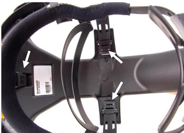
**10.2** Remove the air-duct from the head harness by releasing the three fixing points.
