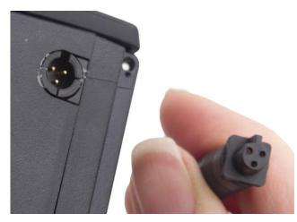
**2.2** Make sure that the pin on the cord's plug is fitted into the groove on the battery.
