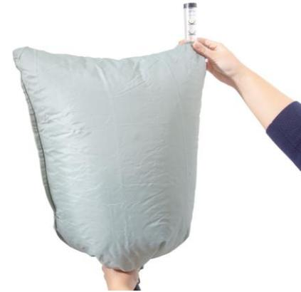
**2.2** Place the head-top in the flow meter and start the fan unit. Grip the bag to seal around the breathing hose. Grip the flow meter tube with the other hand, the tube will point upwards from the bag
