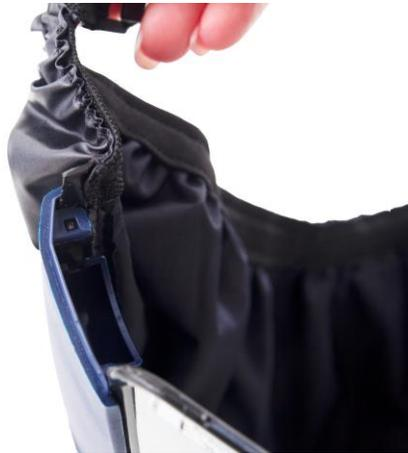
**6.4** Fit the face seal on the inner flange in the lower visor frame. Start at one side, push the pin upwards and control that the lip is fastened in the lower visor frame. Push along the face seal frame so it is securely fastened on the lower visor frame. Control that the pin and lip is fastened on both sides.
