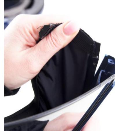
**6.3** Unfasten the face seal by pulling its frame until the pins release from the holes in the visor.
