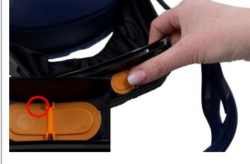
6.3 Press on the new membrane in right position according to the picture. The text "UP" on the membrane should be visible when mounted as shown. Carefully check that the membrane is in contact with the valve seat all round.
